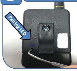
Place GTX Transmitter in Pairing Mode
