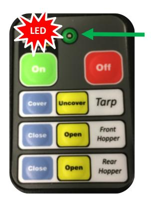
When the transmitter is operating, the RED LED flashes rapidly when a button is pressed. *This Indicates that communication is working between the transmitter and receiver.*
