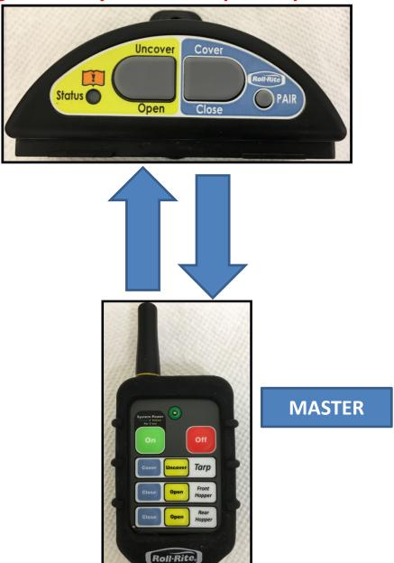
Prior to Pairing a new FIRST REPLACEMENT transmitter to the Receiver, make sure the Transmitter is configured as a MASTER TRANSMITTER, see next section
