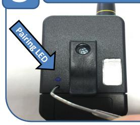
Place GTX Transmitter in Pairing Mode
