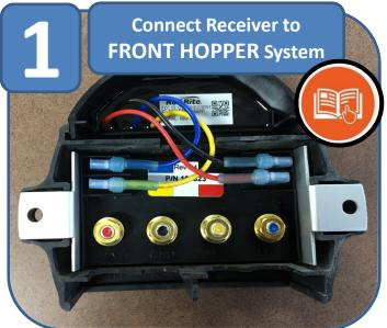
Connect Receiver to FRONT HOPPER System
