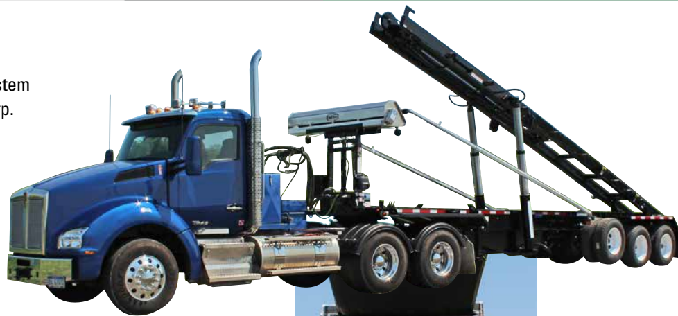
Shown: Extreme duty system includes 2-stage tower. (optional on standard duty systems)
