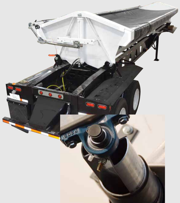
Robust greasable pillow-block bearing on rear arm
